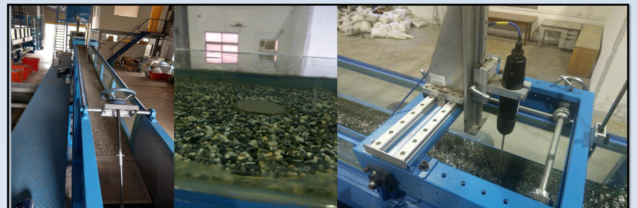
Fig . 1. Photo of the flume, specimens placement area, and the ADV.
